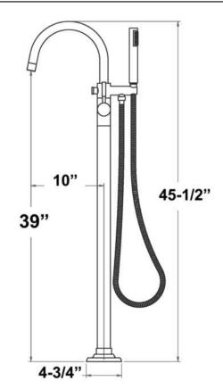
Use on concrete floors requires special installation. We recommend using a plumbing proffessional. Dimensions are nominal and may vary. Dimensions and specifications subject to change without notice.
